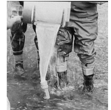
Hess Sampler showing the collection container
